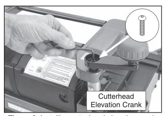
Figure 8. Installing cutterhead elevation crank.
